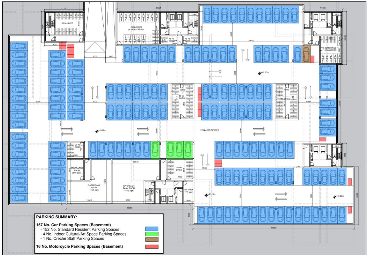
Figure 3-1: Car Parking Facilities (Architectural Drawings by Urban Agency Architects, annotation by PUNCH Consulting Engineers)
