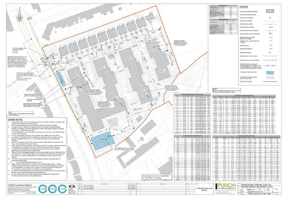
*Figure 13. Proposed ground floor drainage layout*
