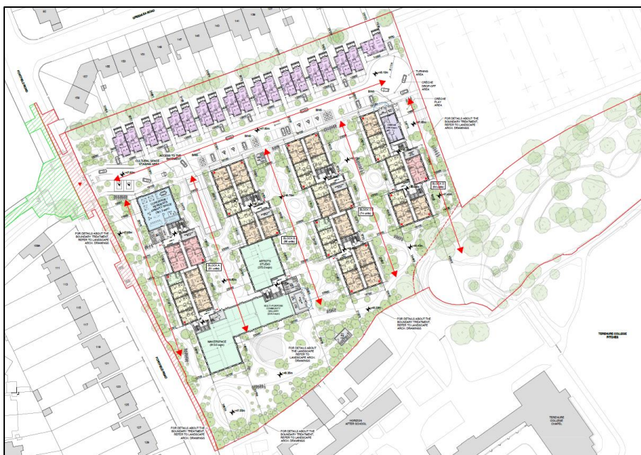
Figure 7: Wind Mitigation Measure – Permeability Paths
