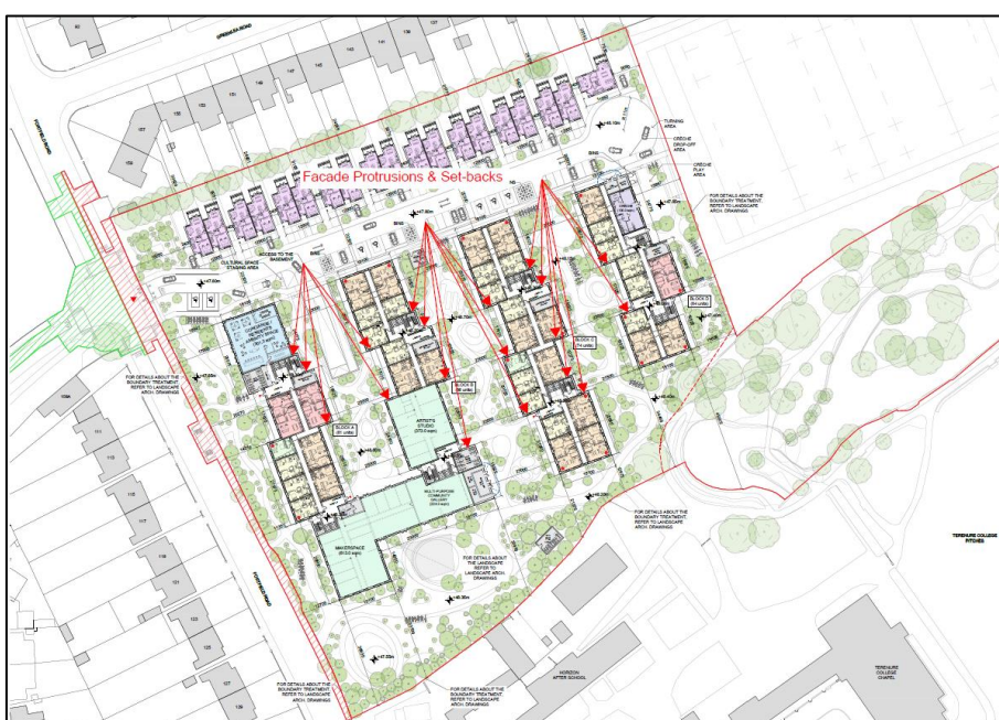
Figure 8: Wind Mitigation Measure – Façade Protrusions and Set-backs
