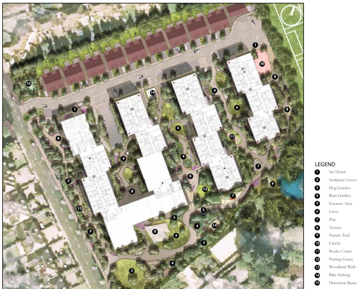
Figure 11: Wind Mitigation Measure - Landscaping Design – Ground Floor
